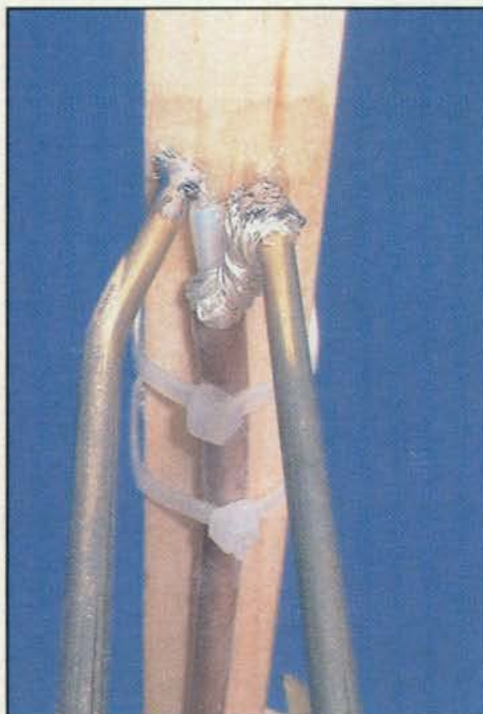
Photo D—Coax attachment on the 2-element Cheap Yagi.
